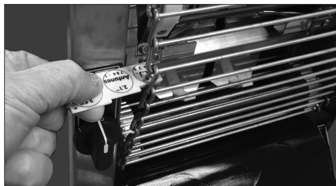
Figure 8. Measuring Conveyor Belt Chain
