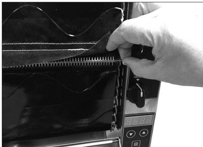
Figure 6. Installing Belt Wrap
